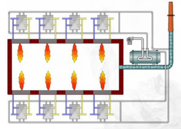
Pre-heating modules are available pre-mounted including pre-heater, high temperature valves, high temperature bypass valves, measurement and control equipment, signal connection box, compressed distribution board for control, pipeline and connection, thermal insulation.
